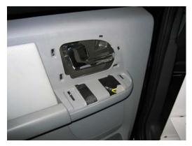
Remove window/lock switch assembly from door
